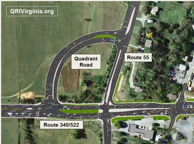
Quadrant Roadway Intersection
